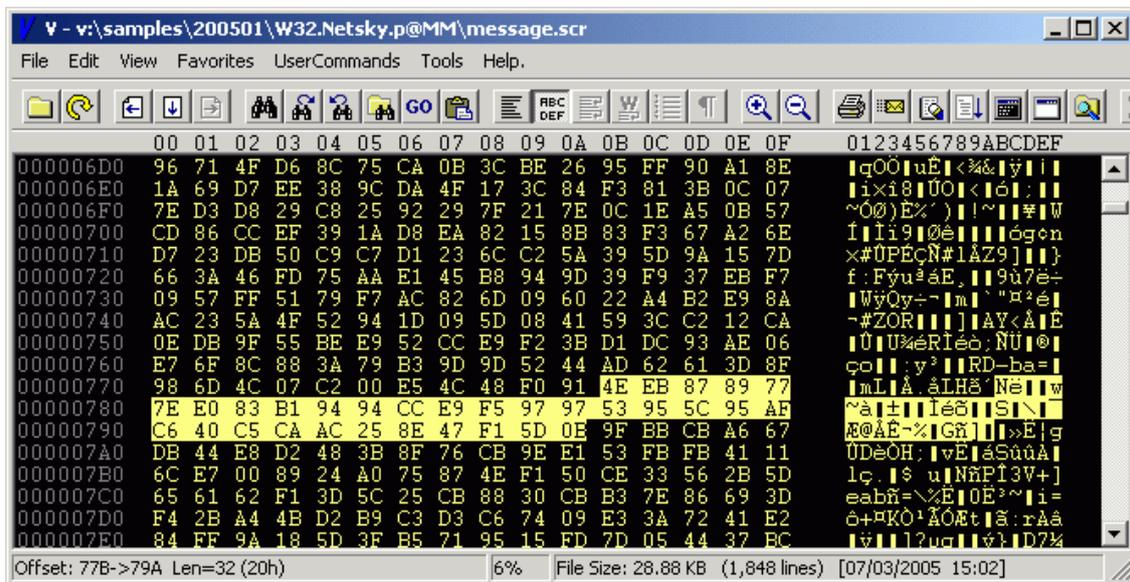
Figure 8: Hex view of a W32/Netsky.p binary sample
